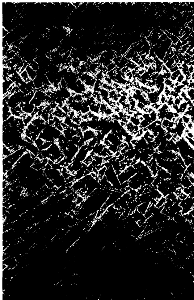
Figure 6 The formation of the smectic S_A -phase in the form of bâtonnets upon cooling of PEAI 7f from the isotropic melt
